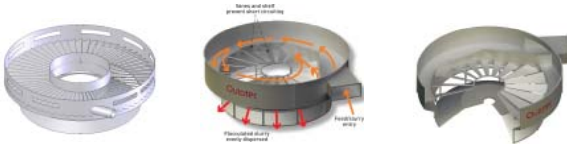
Figure 12: Next Generation Feedwell design (subject to four separate patents)
