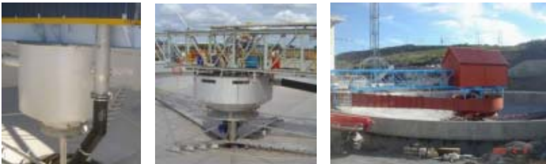
Figures 1, 2 and 3 Low, Medium and High aspect ratio feedwells
