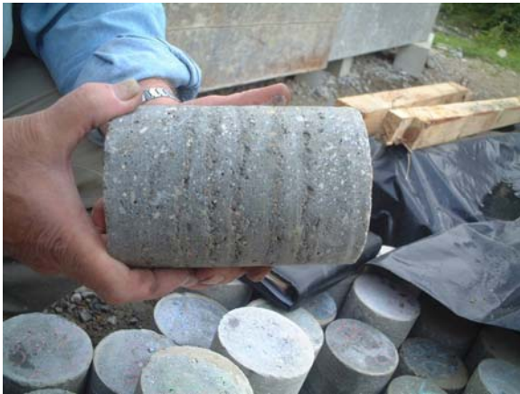
Figure 7 – Pump pulsation can cause pronounced concrete layering
