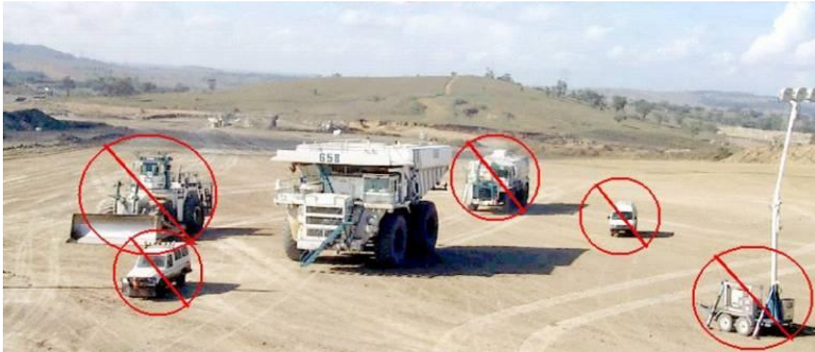
Figure 2 - Large mine equipment has significant blind spots which contribute to vehicle to vehicle collisions.
