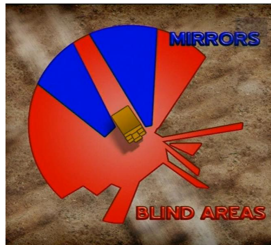
Figure 1 - Red zones indicate blind areas with assistance of rear view mirrors.
